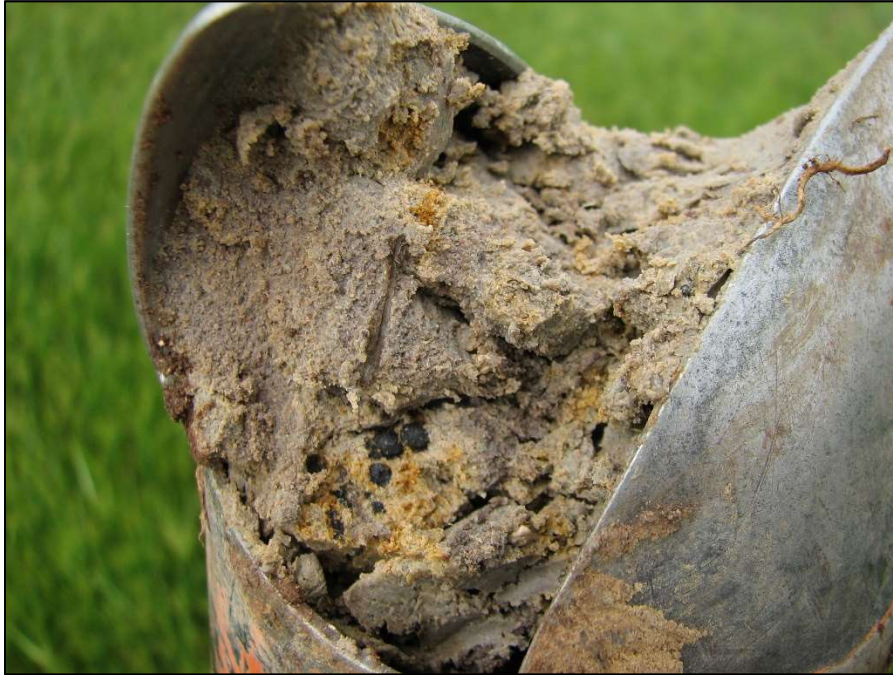
Figure 6: Reduced matrix (grey) with orange and yellow mottles as well as black manganese concretions observable within an augered soil sample from the permanent zone of a hillslope seepage wetland northwest of terrain.
